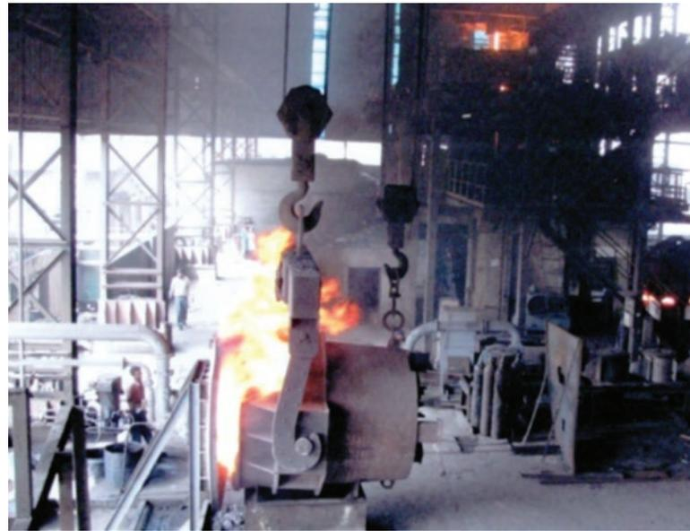
*Crushed steel drums being recycled in a local smelter*
