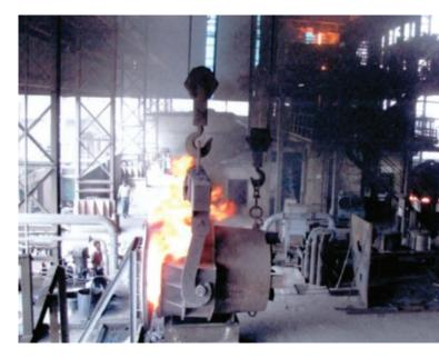
Crushed steel drums being recycled in a local smelter
