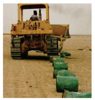
Crushing empty, rinsed drums
