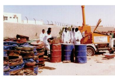
Drum-crushing in progress, using a commercial drumcrushing unit
