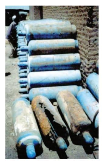
Badly corroded pressure containers
