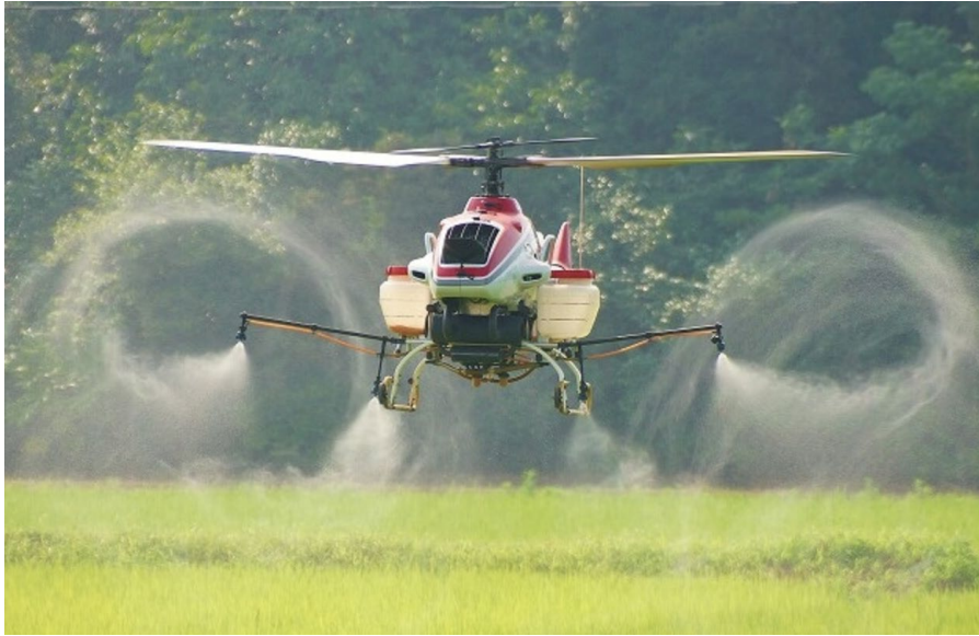
Figure 1: Spray distribution affected by the vortices of a mini-helicopter UAV
