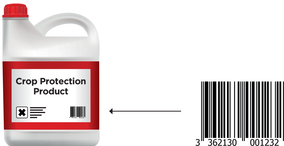
Figure 5: Example of a trade item carrying a GTIN-13 represented in an EAN-13 Bar Code
