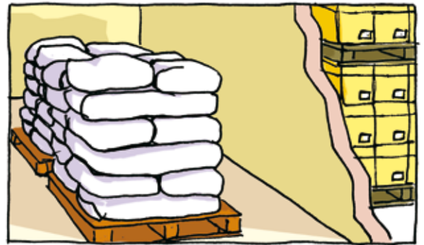
Segregation with a fire wall as a barrier.
