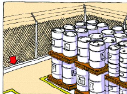
Outdoor storage on a firm base surrounded by a sill
